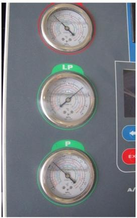
d) Write down the pressure of each gauge, shut down the equipment. After 4 hours, check pressure of the three gauges. If any gauge shows more than 0.1 BAR pressure down, means the pipeline related to that pressure gauge has leakage (refer to pipeline diagram of this manual).
