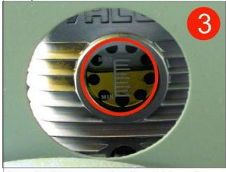
Step3:Observe the liquid level, add oil to the appropriate location
