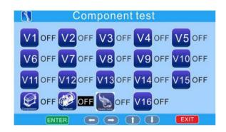
d) In "Component test" page, turn on V1, V5,V17, V9 and V10. Wait until the pressure shown in 3 pressure gauges become equal, turn off the equipment.
