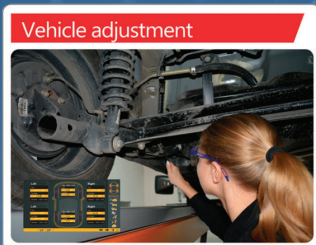
Mount clamps and targets Use the suitable jaw Protect with safe straps
