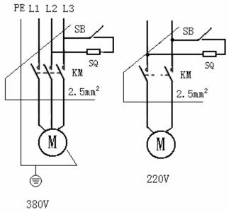
Electrical schematic diagram for **PL4.0-2A**, gantry lifter
