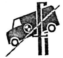
(13) Prevent vehicle from excessive swing in hoist
