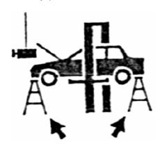
(9) Auxiliary accessories may reduce load capacity (10) Peripheral regions shall be unblocked when Vehicle tilting may occur.
