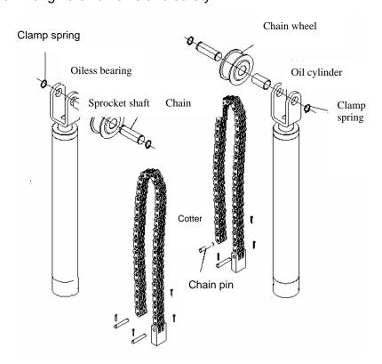
PL4.0-2B, PL4.0-2E, PL4.0-2APL4.0-2ET,PL3.8-2A,PL4.0-SW Installation diagram for chain and oil cylinder of lifter
