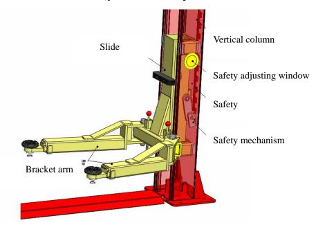
Safety mechanism of, PL4.0-2A, lifter
