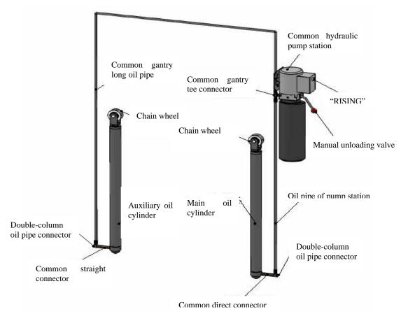
Connection diagram for oil pipe connector of PL4.0-2A lifter
