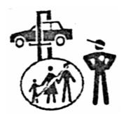
(8) Use safety support at any time when heavy parts are removed or installed
