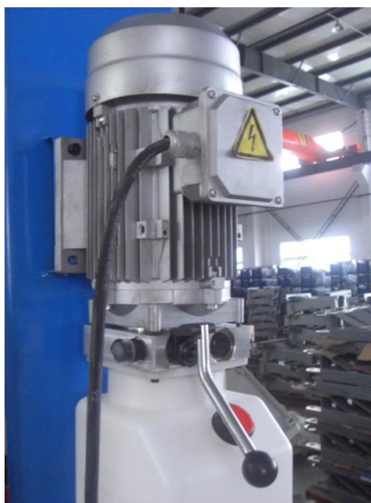
Pump station with control cabinet (Customer optional)
