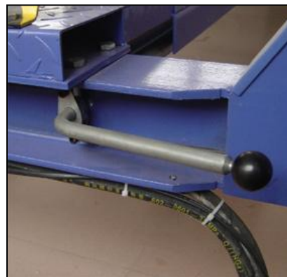
Pump station without control cabinet and lift unlocking method
