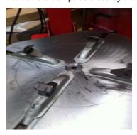
Place the tire on the clamps and press the pedal (3) to open the clamp hand thereby lock the rim. Make sure the rim is firmly fixed to the clamps.
