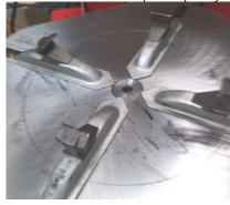
Warning: splitter with the clamps in the open position can be extremely dangerous for operator's hands; during the splitting operations never touch the side of the tire.
