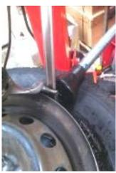
WARNING: In order not to damage the inner tube, if there is one, it is advisable to carry out this operation with the valve 10cm to the right of the mounting head.
