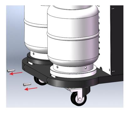
Remove the two lock bolts, to release load cells of the two tanks, and to make them ready to work. *Warning:*
