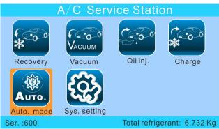
In auto. Mode, the machine makes recovery, vacuum, oil injection and refrigerant charge in sequence automatically, with data preset by users.
