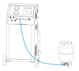
Through tank fittings, connect either HP or LP hose with external refrigerant R134a or HFO-1234yf, and turn on the machine, select "Tank fill" function, set tank fill amount to fill R134a or HFO-1234yf tank with refrigerant.
