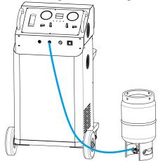
Connect either HP or LP hose with external refrigerant R134a or HFO-1234yf tank, and turn on the machine, select corresponding refrigerant type, run recovery to fill equipment with refrigerant. After one refrigerant tank is filled, fill other tank with its corresponding refrigerant.
