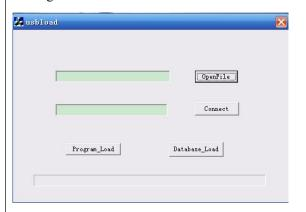
Click "Program\_load" for main program update, or click "Database\_load" for database update, the machine displays the following:
