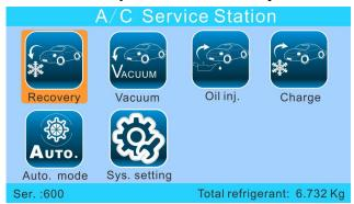
The recovery process recovers the refrigerant from vehicle A/C system, until a vacuum is achieved in the vehicle A/C system. Moisture, oil and foreign particles are separated from the refrigerant before it is stored in the internal refrigerant cylinder.
