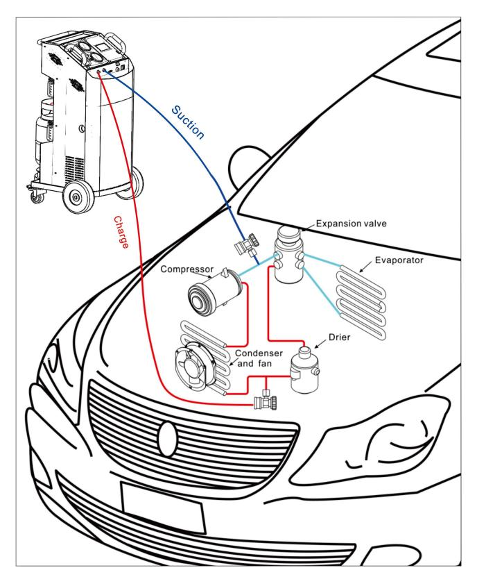
Warning: Except the situations clearly stated in the manual, during recovery and all other equipment operations, please maintain the vehicle engine and A/C off, otherwise unexpected damages may be caused.
