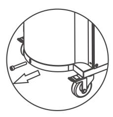
Remove the bolt that fix tank platform with chassis, to release tank load cell.
