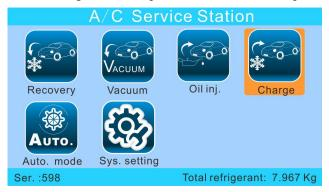
You can manually set charge amount with volume, or select "Charge by database" to set charge amount by car make and model.
