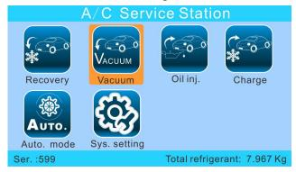
The Vacuum process evacuates system, and makes system ready for oil injection and refrigerant charge. Although it is up to users to determine vacuum time, a longer vacuum process is recommended.
