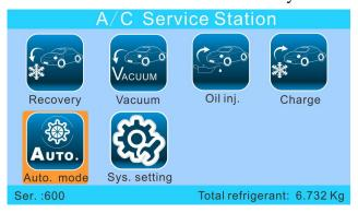
In auto. Mode, the machine makes recovery, vacuum, oil injection and refrigerant charge in sequence automatically, with data preset by users.
